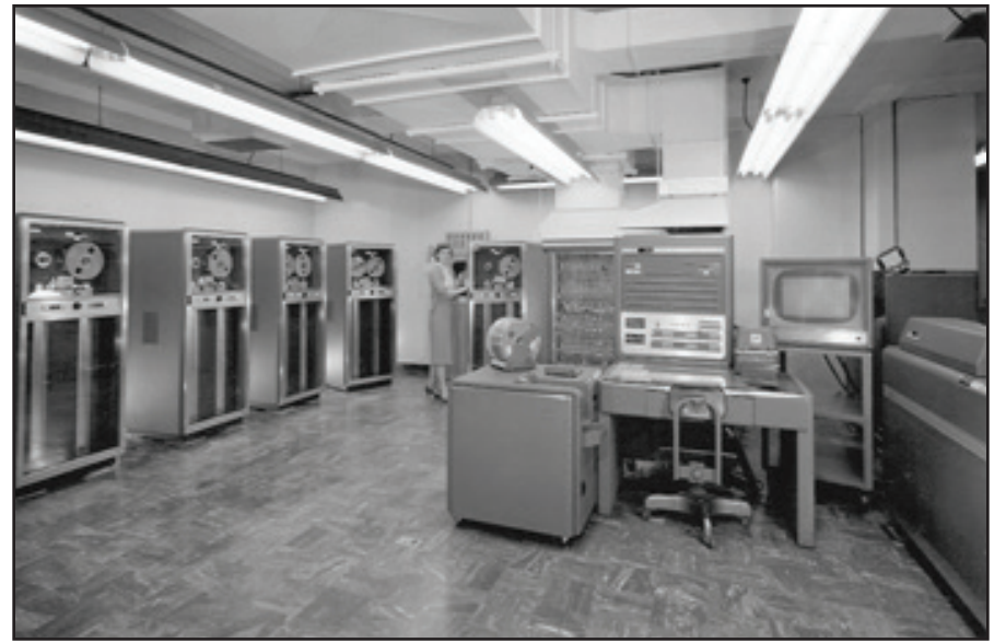
Figure 1. The mainframe of an IBM 704: a state-of-the-art, high-speed digital computer in the late 1950s. Figure courtesy of Lawrence Livermore National Laboratory via Wikimedia Commons.
